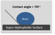
Nano4Diamond boasts a water contact angle of 150°. Contact angles of over 120° are considered Super-Hydrophobic
